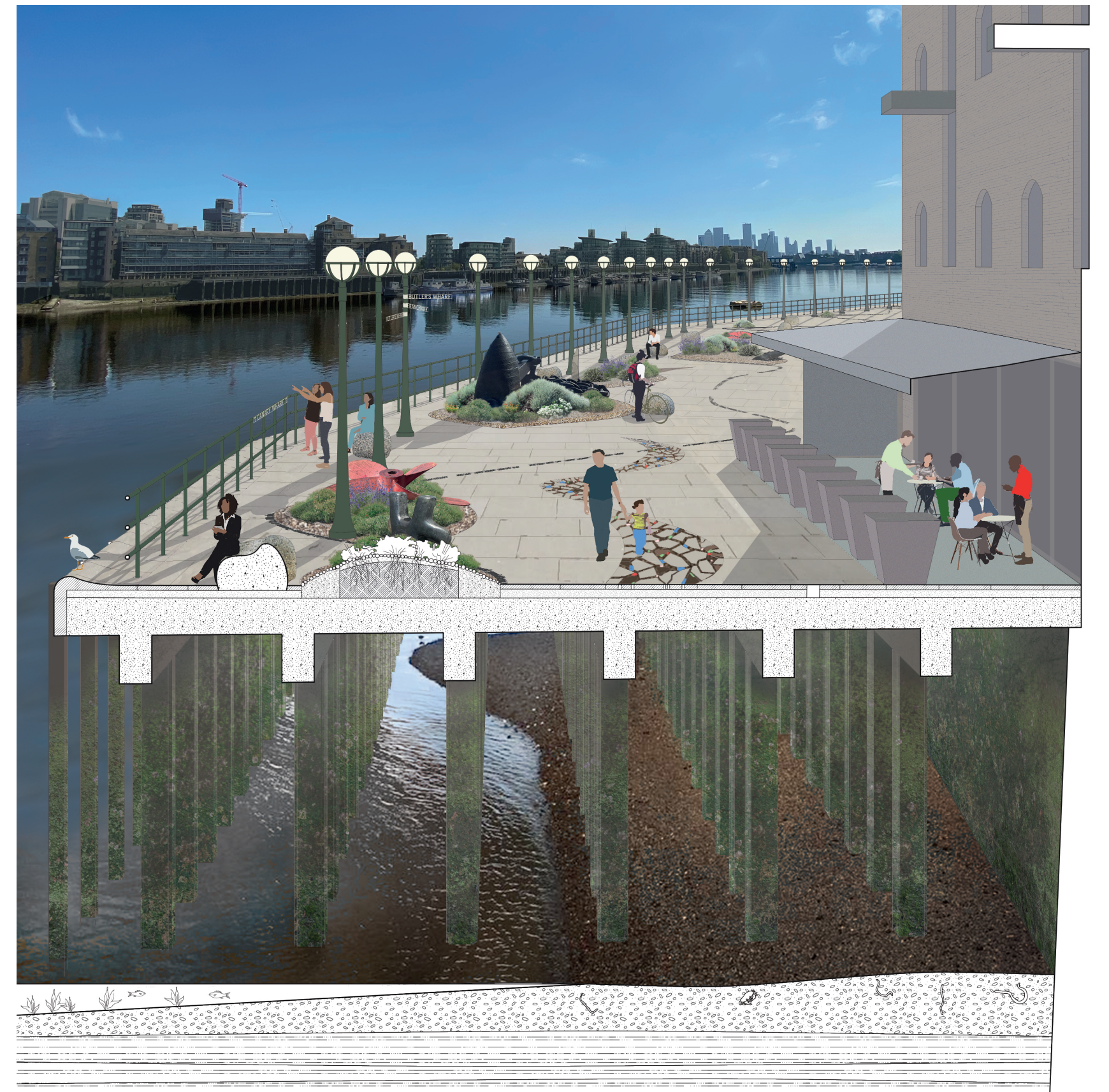
Section perspective showing the relationship between the river bed and new treatments to the jetty
